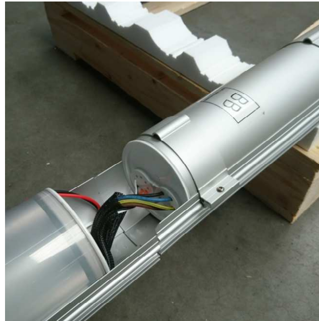
Picture 2: Place the connectors and the sealing disk in the aluminum housing. Make sure the sealing disk closes the housing properly to ensure water resistance.
