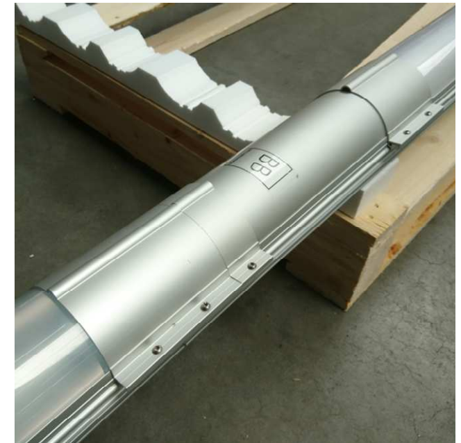
Picture 3: Slide the cover onto the transition of the two fixtures and fasten the torx screws.
