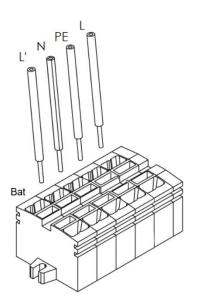
L' - a switchable phase that should be connected from the L phase
