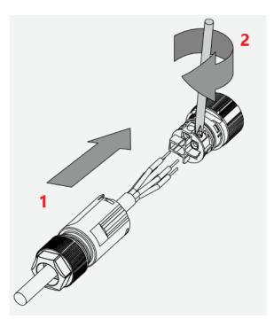
• assembly both parts of the plug, as presented on the scheme below:
